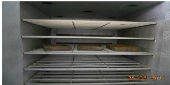
**Picture 1: Laboratory Furnace for Removing Humidity of Nickel Ore in New Smelter of Ferronickel, Drenas**
